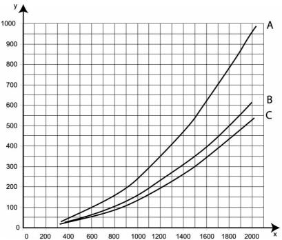
0 200 400 600 800 1000 1200 1400 1600 1800 2000 X X-axis: m³/h Y-axis: Static Pa A: Extension arm bent 40° (to its limit). B: Extension arm bent 90°. C Extension arm is straight.
